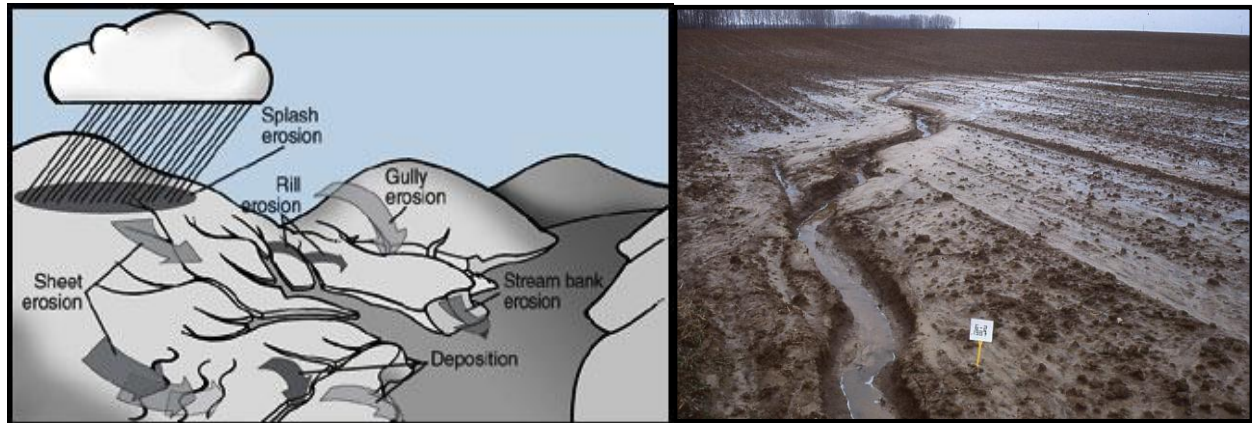
Figure 2.2 Type of Erosion
