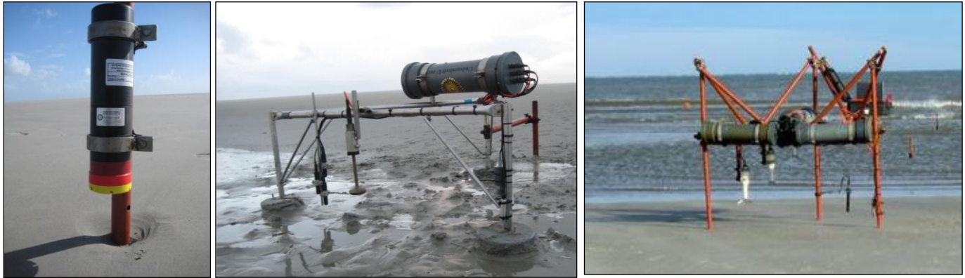
Figure 2.4: (left) An OSSI, (centre) a miniframe with f.l.t.r. OBSs , an EMF, a floater and a pressure sensor. (right) the Truc Vert frame with f.l.t.r. three ADVs, the OBS-array, and a pressure transducer and floater on the most right 'leg'.
