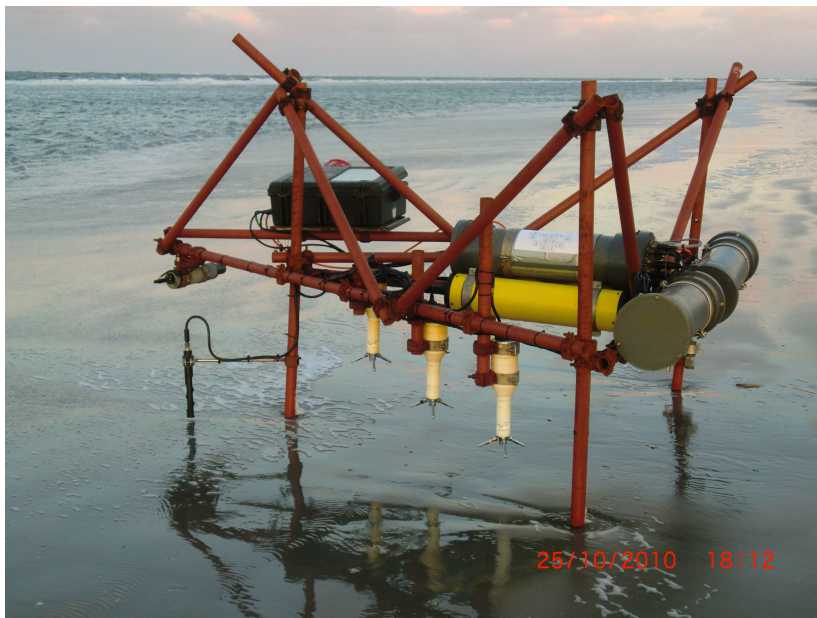
Figure 4.2 Instrumented rig deployed at the neap low-tide water level during the Ameland 2010 field experiment.
