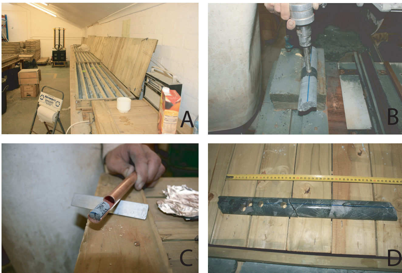
FIGURE 3. Impression of sampling the drilling cores in Cape Town. A) The wooden boxes in which the cores (already cut in half) were transported and stored. B) Vertical drilling of a core-piece on the wooden construction on the saw-table. At the right-top of the photo the saw is visible. C) Example of a small core sample. D) Part of a core after drilling of samples for this study.
