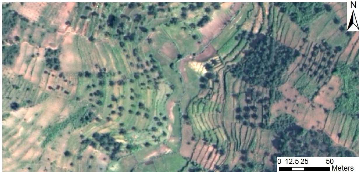
Figure 6.1: Similar bench terraces on two sides of a valley running from north to south in the Sunga study area. The terraces in the east are more clearly visible due to the shadows of the terraces. NB: The sun is positioned in the east.
