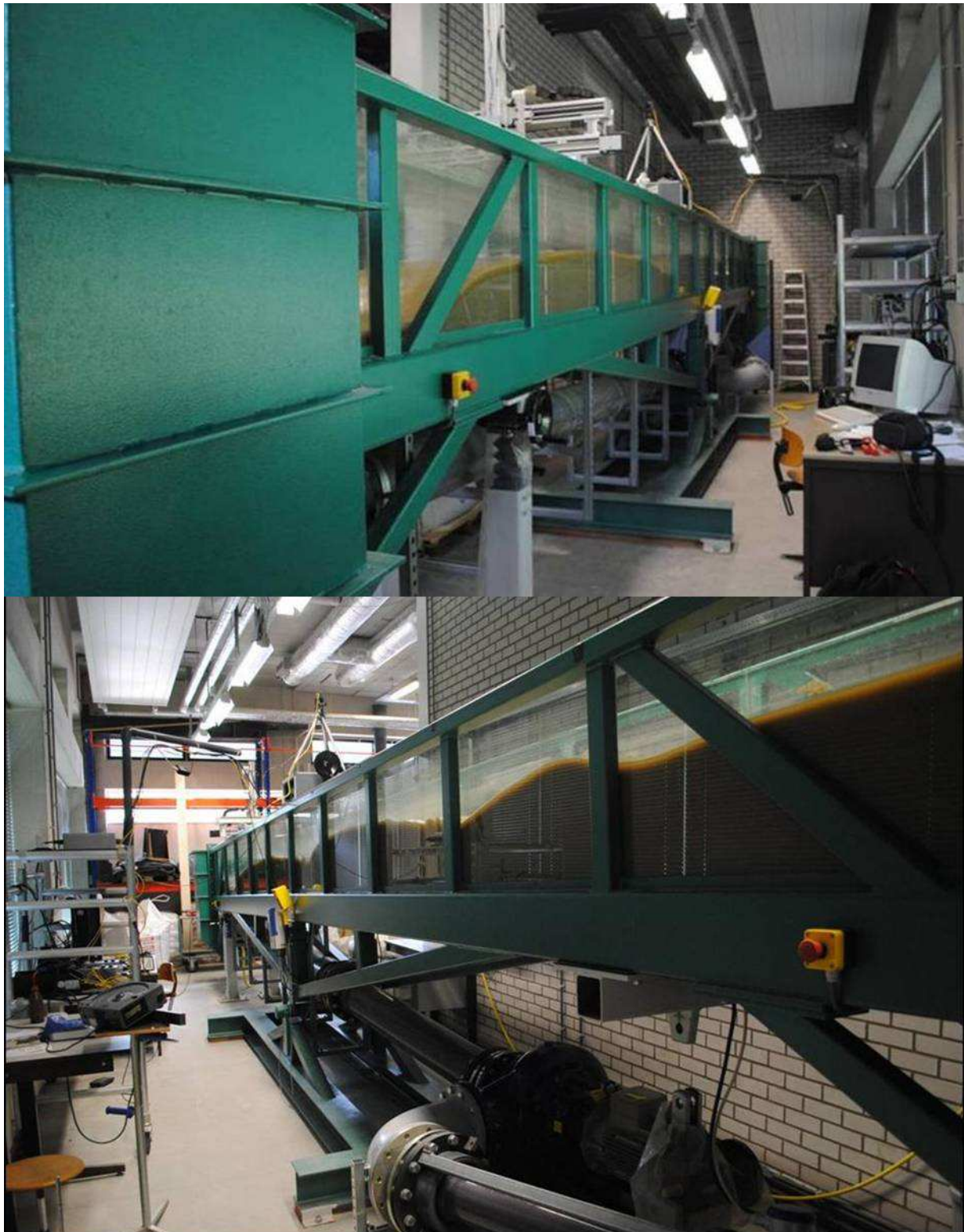
Figure 6 Flume used in the experiments during a run establishing cyclic steps, the vertical bars are spaced at 1 meter
