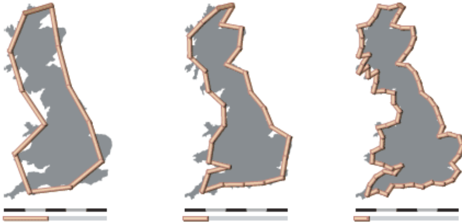
Figure 1.4: Measuring distance using fractional dimension with (from left) a 200Km, a 100Km and a 50Km unit.
