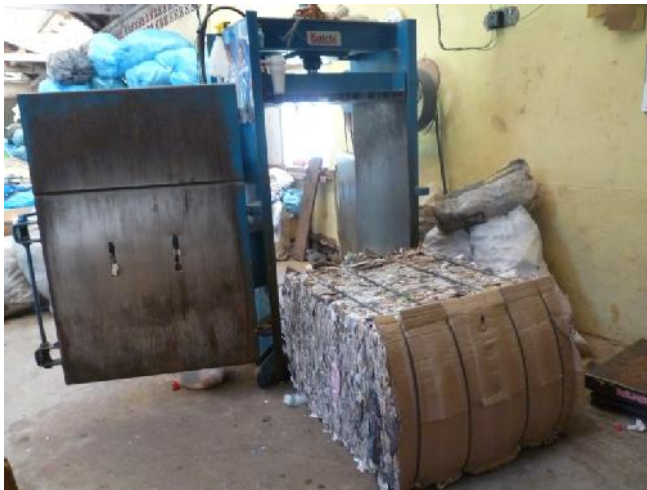
Picture 4.3 – Pressing machine to pack materials
