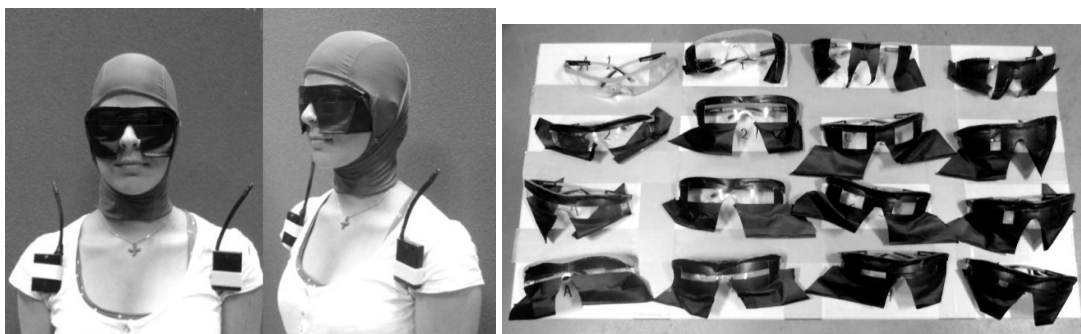
Figure 1. An example of the goggles worn together with a forage cap and the wordviz leds (However, this photograph is without the xsens motion capture suit). On the right all different goggles are displayed.
