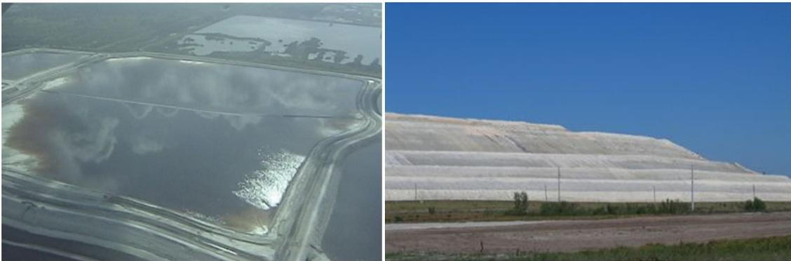
Figure 1.1. Phosphogypsum stacks near a phosphate fertilizer industrial plant in Polk County, Florida [DEP].
