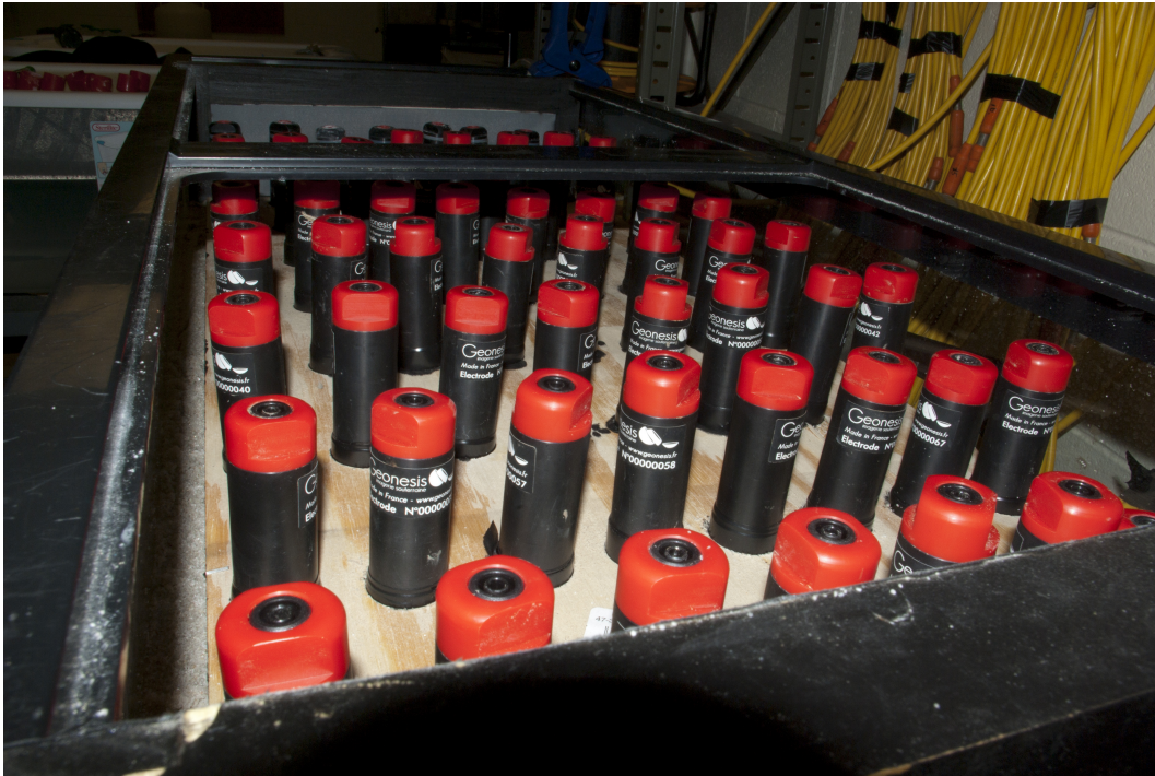
Figure 5.5: The electrodes that were used for the DC resistivity and IP measurements were placed 2 cm into the sand aquifer and were kept in place by a plywood board.
