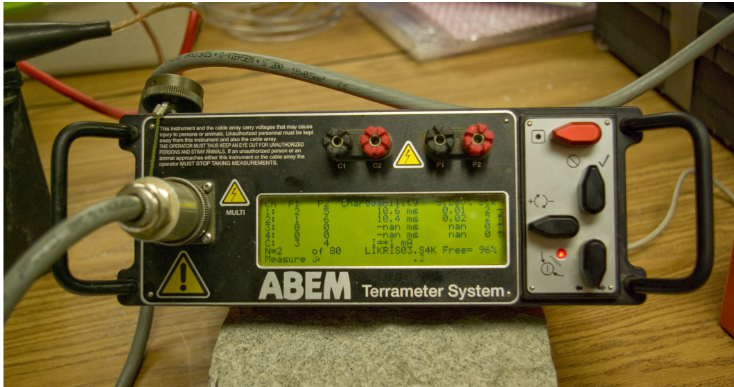
Figure 5.3: The ABEM Terrameter SAS 4000 system in action. The grey cable on the left is connected to a switcher box (also available from ABEM) which in also connected to two cables (visible in Figure 5.6) with 32 electrodes each.
