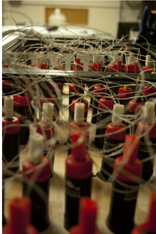
Figure 5.6: The electrodes were connected to the ABEM switcher box by two customly designed cables, that have 32 electrode connectors each.
