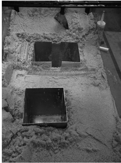
Figure 3.2: A view of how the sand columns were constructed, using metal shields to prevent the sides to collapse in unstable saturated sand.
