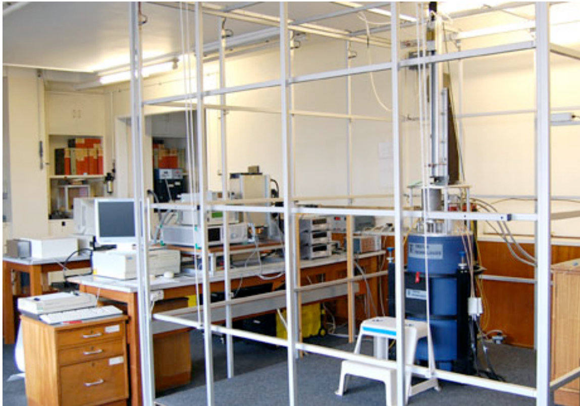
Fig. 5.5 The automated microwave system at the University of Liverpool, combined with a Tristan Technologies liquid helium cooled SQUID magnetometer with a cryocooler. (Source: http://www.liv.ac.uk/earth/geomagnetism/facilities.htm .)
