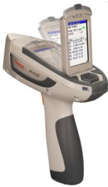
Figure 4. Thermo Fisher Scientific Niton® XL3t-600 handheld XRF analyser (LearnXRF, 2011).
