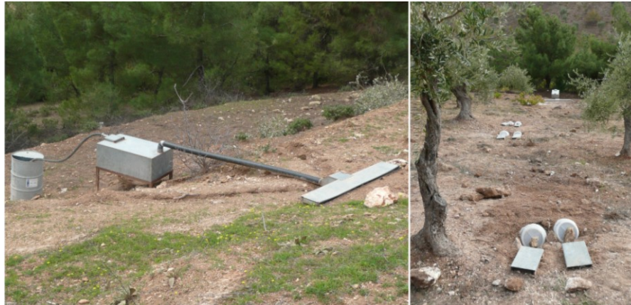
Figure 2-5 The experimental set-up for surface runoff and soil loss measurements in field 3. Left: Gerlach trough set-up Right: Small collectors. Photos: E.H. van der Zanden
