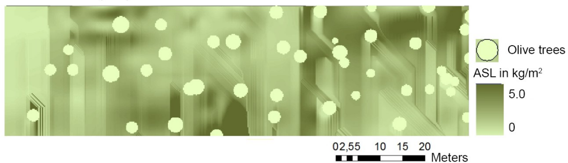
Figure 3-6 RMMF model output: runoff and annual soil loss maps for field 3, including olive tree positions and ACED erosive areas.
