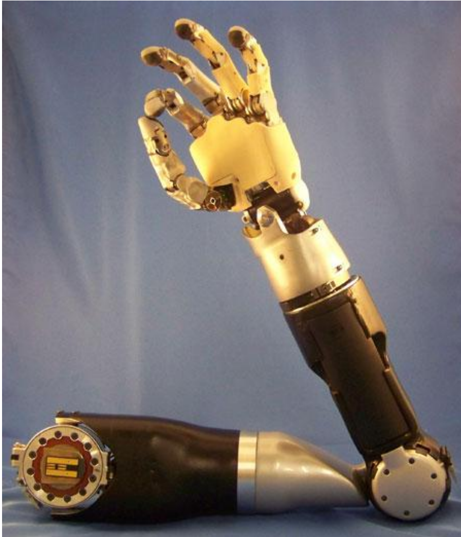
The modular prosthetic limb, waiting human trials.
