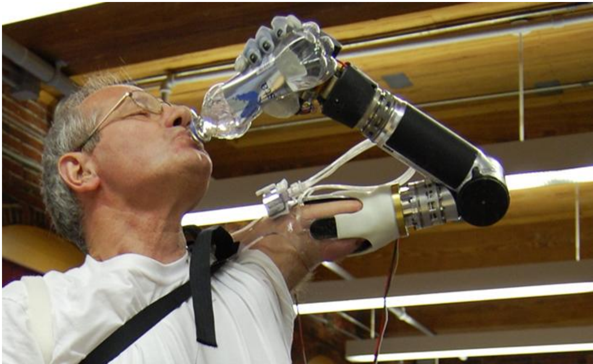
Man wearing the latest myoelectric deka arm, drinking water.
