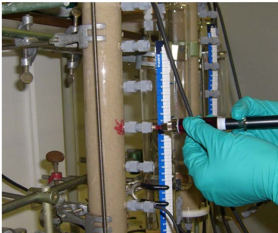
Fig 6: Injection of toluene in the column.
