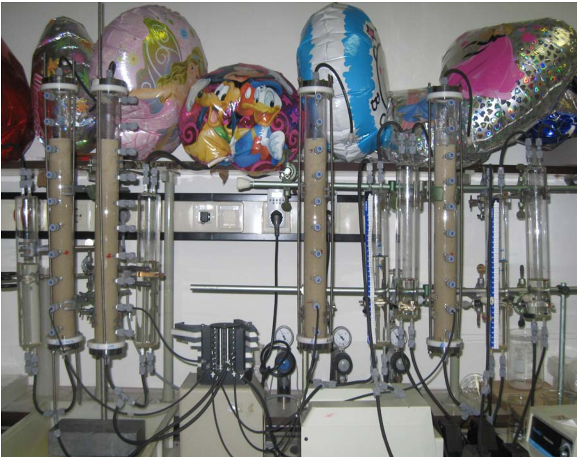
Fig 5: Picture of the column setups with the static water level (left) and dynamic water level (right).
