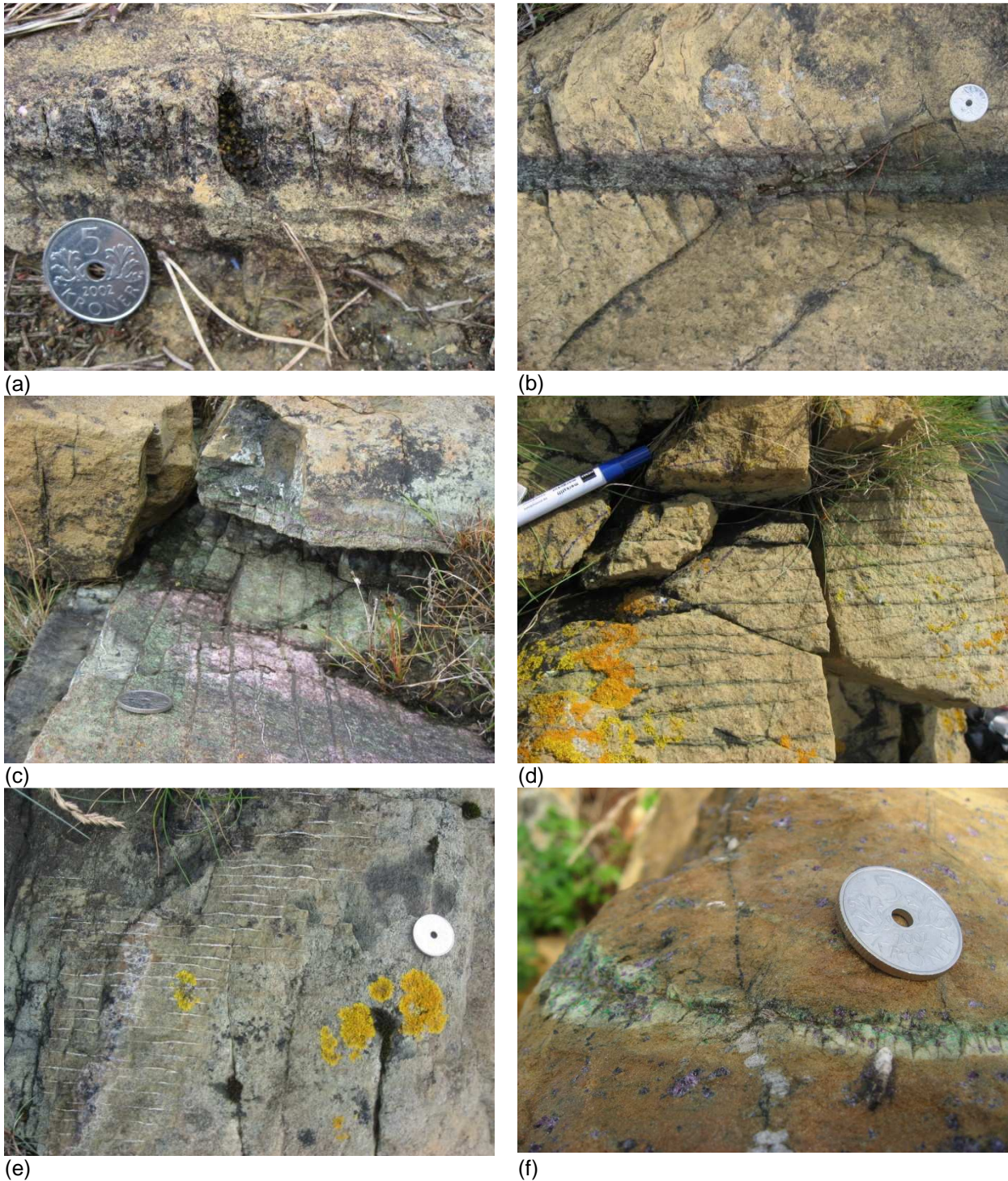
Figure 2-10: (a) Regular fracture pattern in pyroxenite layer perpendicular to the layer. (b) Fracture pattern in pyroxenite layer at slight angle. (Raudhaugene); (c)-(e) Top view of pyroxenite layer with one set of parallel fractures; (f) Thin pyroxenite layer with fractures perpendicular to layer, but most likely not parallel to each other. (Ugelvik)
