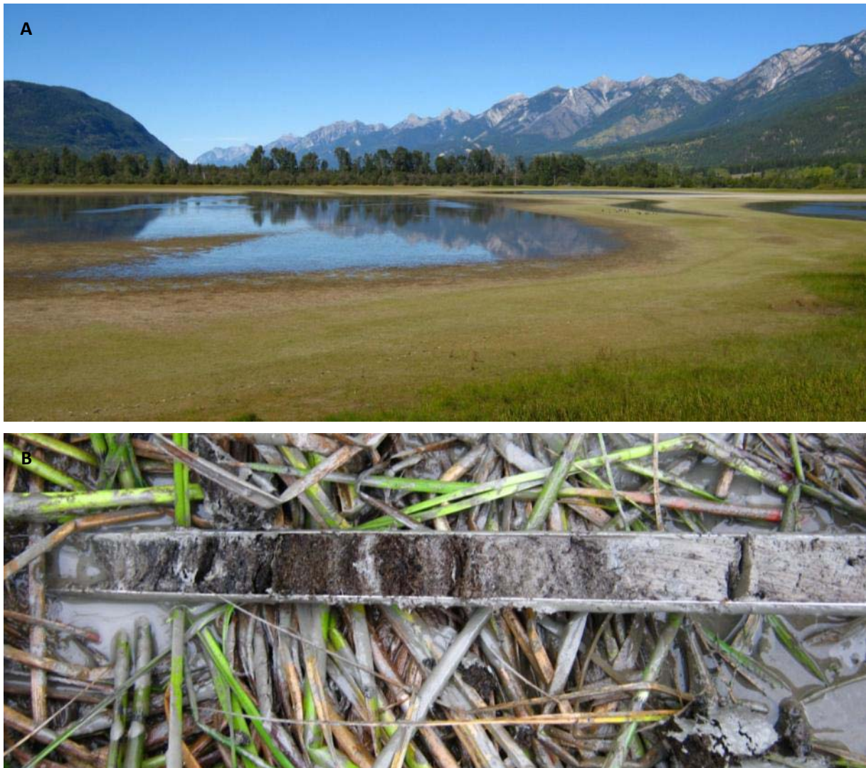
Figure 10. A: Floodbasin partly filled with water. This floodbasin is located just downstream of the elevated cross-valley road at Spillimacheen. B: Thinly laminated organic and clastic mud. Core is taken with a gouge at boring 044 in the transect at Parson.
