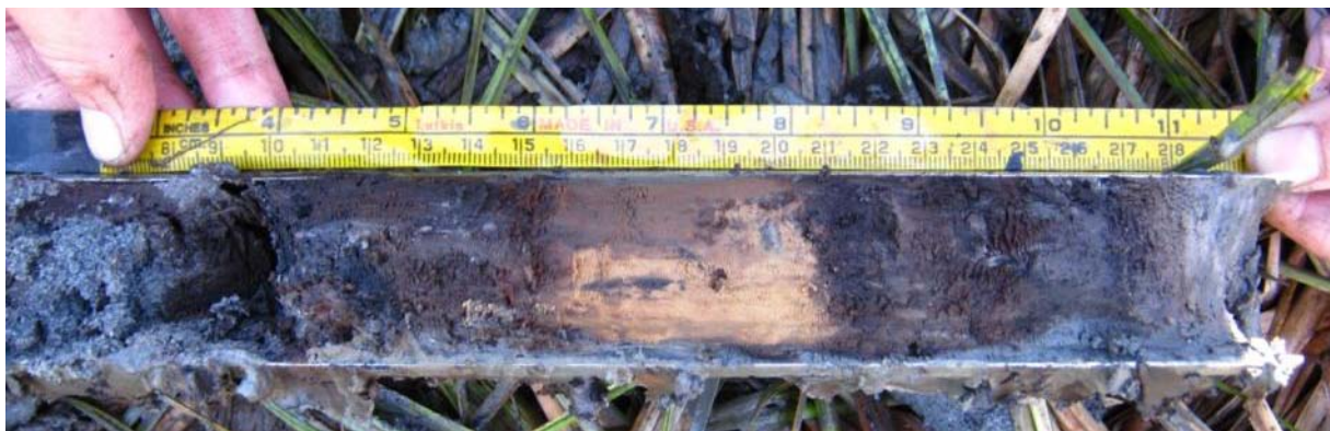
Figure 6. Gouge used for taking samples for dating of macrofossils. Exact depth measured using a measuring tape.
