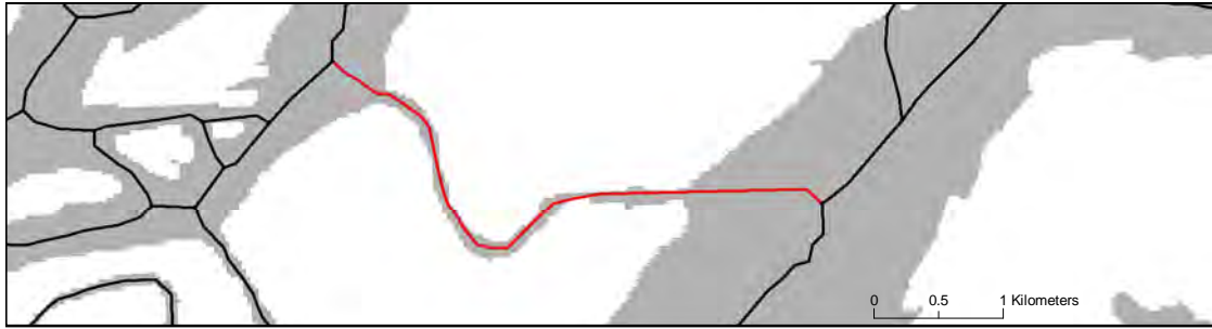
Figure 5.1 Overestimation of channel width when a narrow channel is connected to a wide channel. At both ends of the highlighted channel (in red), the large distance to the nearest bank causes the width of this channel to be too high. This effect is larger for shorter channels.
