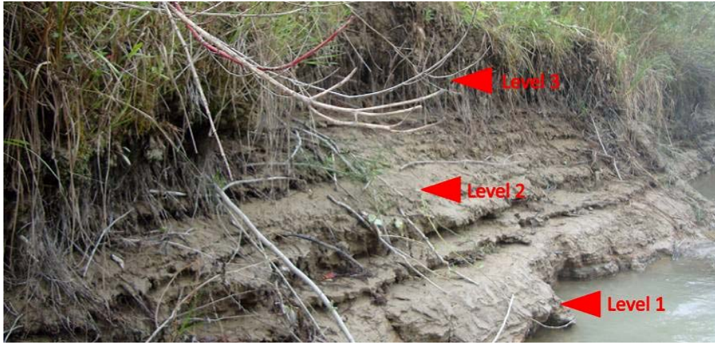
Fig. 3.3: Location of the different shear vane measurement levels.
