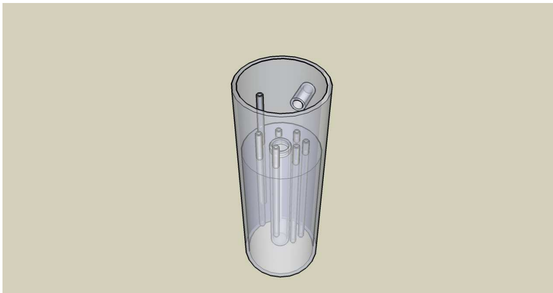
Figure 7 – the organ type infiltration well, with a larger pipe present in the middle
