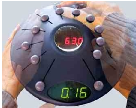
Figure 13: The alarm clock designed by Wensveen et al. (2004) . Each slider can create a different sound. All sliders together form a variety of patterns, (a)symmetrical or (dis)satisfying, depending on the user and their mood.
