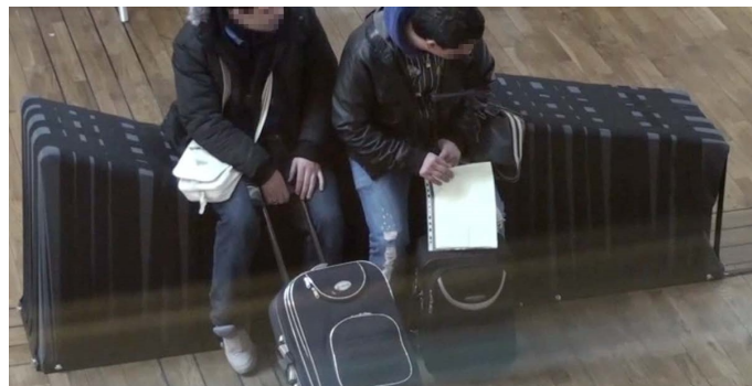
Figure 15: The coMotion Bench, created by Rasmussen et al. (2013), is a shape-changing bench that can change heights in different ways. When someone sits down on the bench, in time it will provide a small vertical push under the person.
