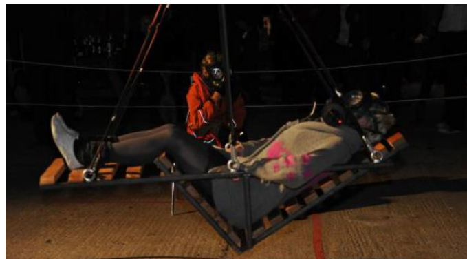
Figure 20: Breathless, created by Benford et al. (2012) , is a swing that moves according to a user's breath. The user puts on a gas mask with embedded breath sensors. When the user inhales, the swing will pull backwards and when the user exhales, the swing will push forwards.
