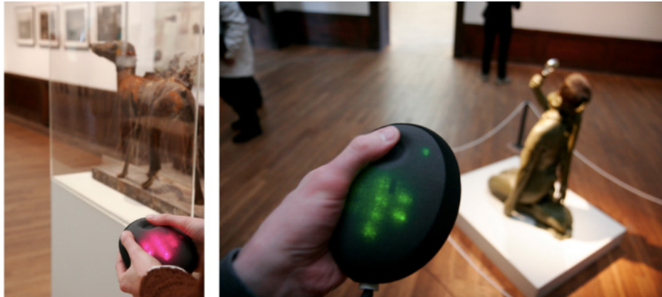
Figure 9: The Lega, created by Laaksolahti et al. (2010) , is a hand held device that lets visitors to an art gallery share their experience via physical traces such as light and vibration. By touching or moving the devices, users can create expressions that are left at the location.
