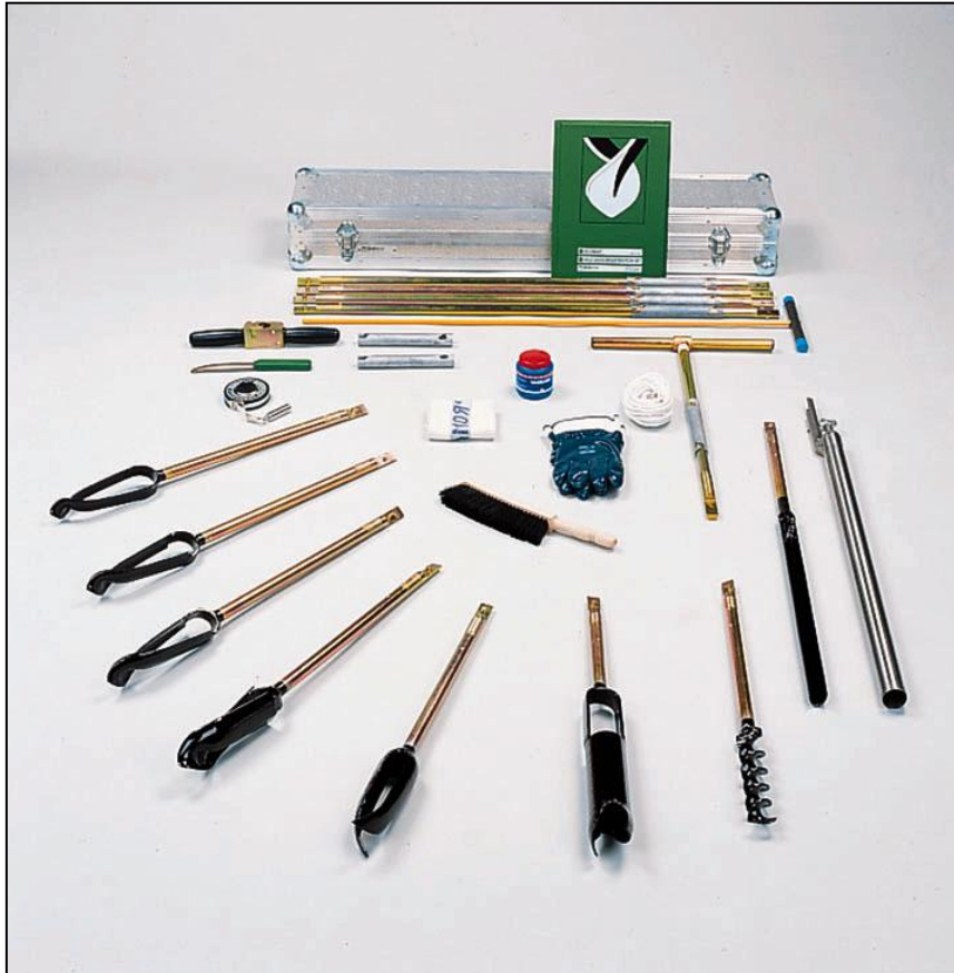
Figure 11 Edelman coring equipment, including, rods, corer and gauge (Berendsen & Stouthamer, 2001).
