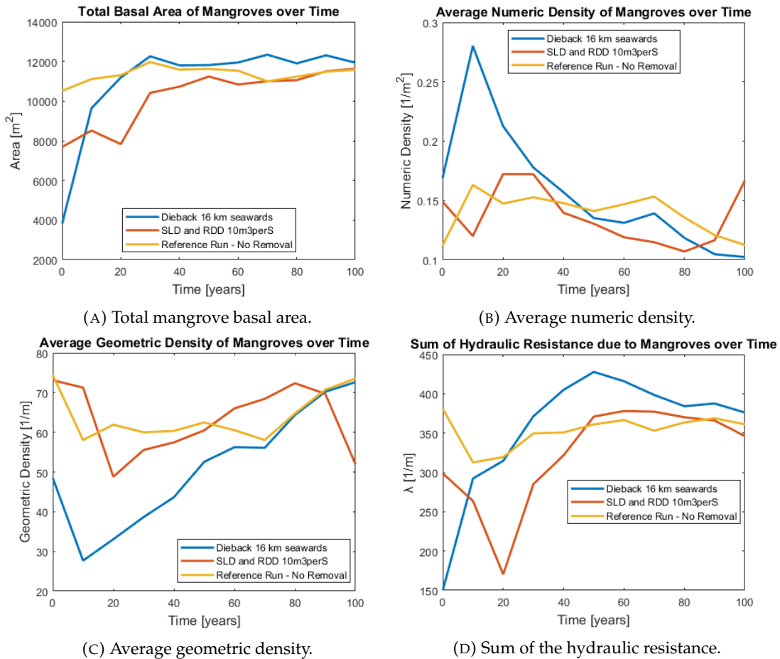
FIGURE 6.23: Mangrove characteristics over the 100 years of recovery over the whole domain including (A) Mangrove tree total basal area, (B) average numeric density, (C) average geometric density and (B) hydraulic resistance on the basis of lamda over the 100 years recovery of the three scenarios.
