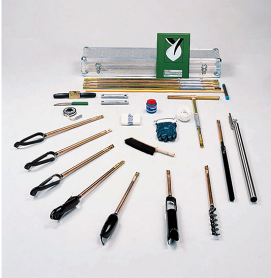
Figure 3.5a: prospection coring material (after: www.eikelkamp.nl )
