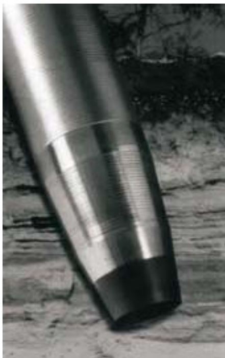
Figure 3.6a: picture of the Begemann steel outer barrel with cutting edge (after: Deltares 2009)
