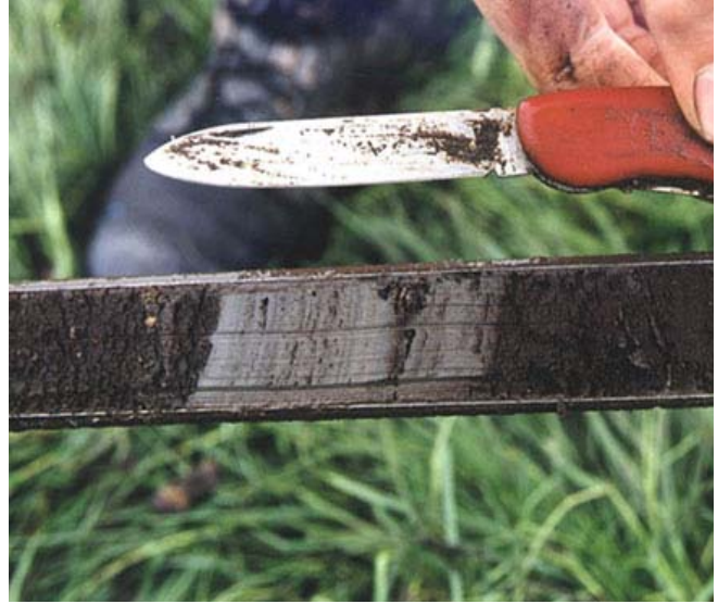
Figure 3.5b: Example of sampling with the simple hand gauge (after: coring methods )
