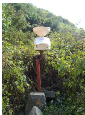
Figure 3.4: The infield installed tipping bucket at the reservoir location (Gortmaker, 2010)
