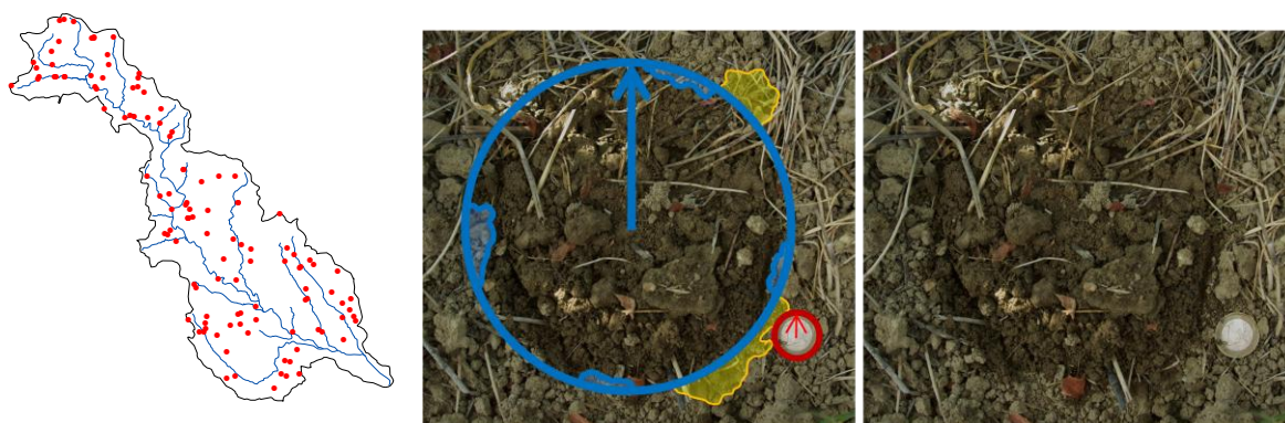
Figure 3.2: a) Locations of the infield observations b) Measuring the wetted perimeter c) Infiltration location after 20min of water supplying
