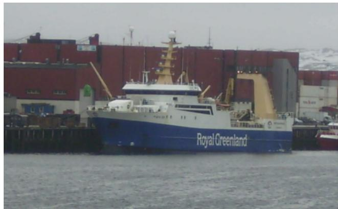
families. When the nets are hauled in, the onboard factory facilities select, sort, cook and pack the catches. Subsequently the packages of shrimp are transported to the big cargo compartment, stretching from bow to stern. When the vessels return to the harbour with a maximum load of 800 tons, unloading and resupplying takes about 24 hours, conducted by a separate land-based unloading crew<sup>58</sup>.
