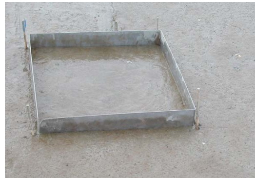
Figure 8: 50 x 50 cm tray (patch) in which the two labels in artificial sea water are added.
