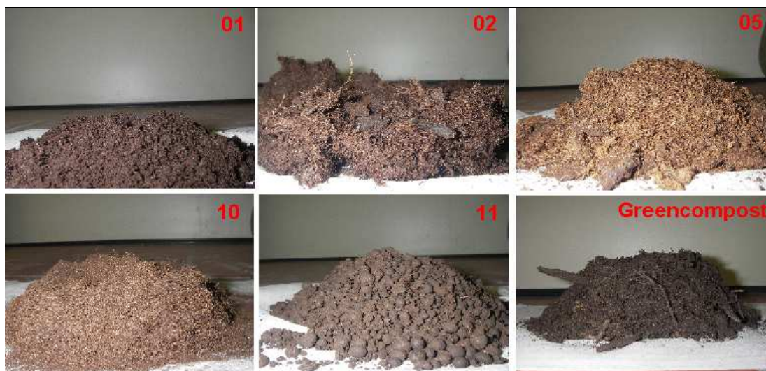
Figure 4.2 The adsorption materials: 01) crumbly, fine material which is used as garden soil. 02) hairy, fibre like material. 05) fine to coarse material, richer in fibre content than 01. 10) very fine dusty material. 11) grain structure with a diameter of approximately 5 mm (used in aquaria). Green compost) Green compost with coarser parts from twigs and such.
