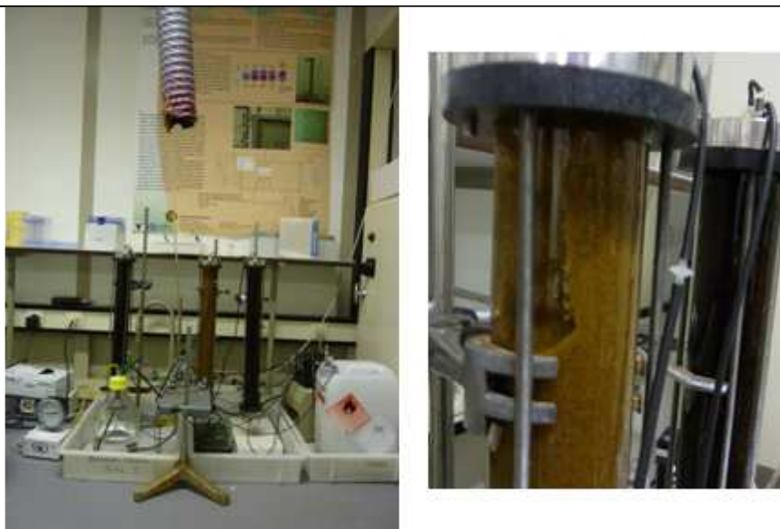
Figure 4.6 Picture of the column experiment set-up and the enclosed air in the sand column.
