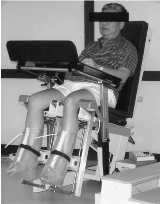
Figure 1. Setup for the assessment of knee joint proprioception, showing the measurement chair control mechanism, air splints, and footrest (the moving component of the instrument).
