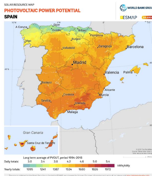
Figure 9. Solar energy resources in Spain, as specific photovoltaic output per kWp and per day (Solar resource maps and GIS data, n.d.).
