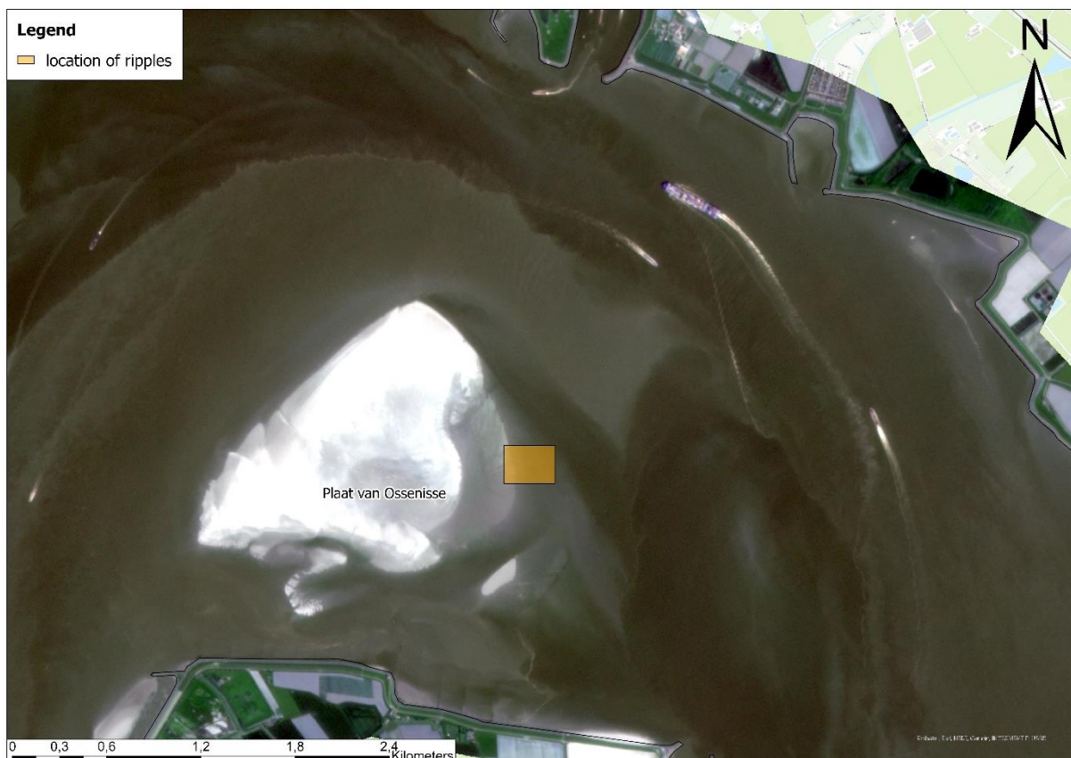
Figure 6: Sediment concentration at the water surface of the Westerschelde, showing indications in sediment concentration visible at the water surface for flow separation on the eastern side of the large bar. In orange the location of Figure 15 a) Image: 2023-05-31 planet imagery “Imagery © 2023 Planet Labs”.
