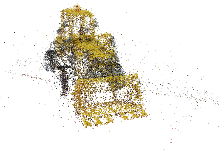
Figure 3.10: Point cloud of OOI with floor removed. Note that the bottom of the tracks on the bulldozer has also been mostly removed.
