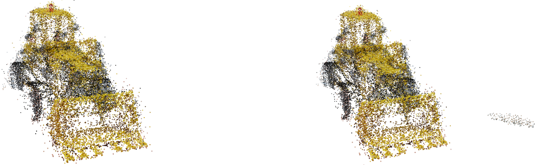
(a) Denoising of OOI using DBSCAN after floor separation.
