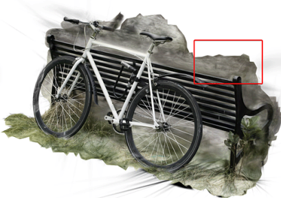
Figure 4.7: View inconsistencies in the 3DGS reconstruction due to undersegmentation in the meshing process. The black Gaussians and the areas marked with red arrows/rectangles showcase the view inconsistencies.
