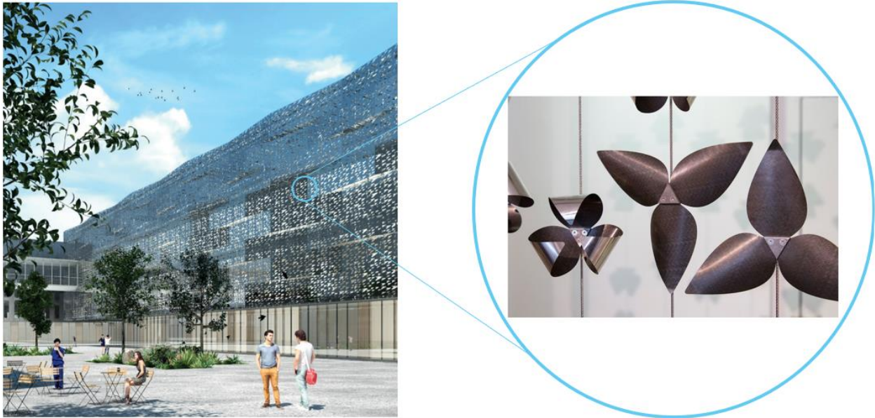
Figure 21 - Left: Simulated image of the IARC façade with Pho'liage adaptive shading, where a pilot was to be tested in 2022. Right: The tripolar prototype of Pho'liage made of TBM that respond to heat changes while maintaining rigidity, and are resilient when exposed to wind loads and pollution. They are now also investigating biopolymers to reduce the amount of TBMs required in the curving petals. Image credit: ArtBuild ©.
