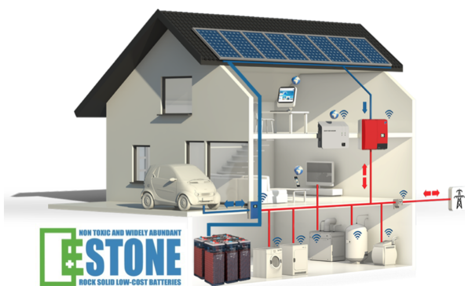
FIGURE 1.1: Envisaged residential application of E-stone batteries in combination with solar panels connected to the grid (Used in approval from E.STONE Batteries).
