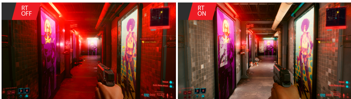
Figure 2: Comparison of ray tracing vs the standard lighting implementation in Cyberpunk [1]. In the right image, we can see much better shadows and reflections on the floor and walls.
