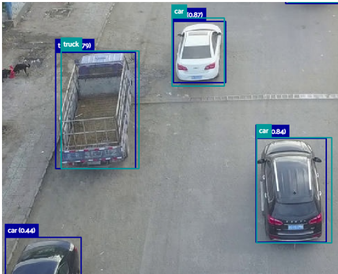
Fig. 12. Early cut-off of annotations in Visdrone-VID. Cyan is the annotated label, while blue is the model prediction.
