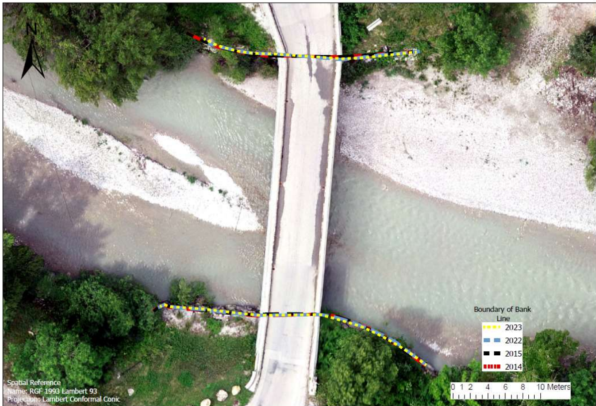
Figure 38 : Bank lines at the location of bridge in every year , represented on Orthomosaic of 2023
