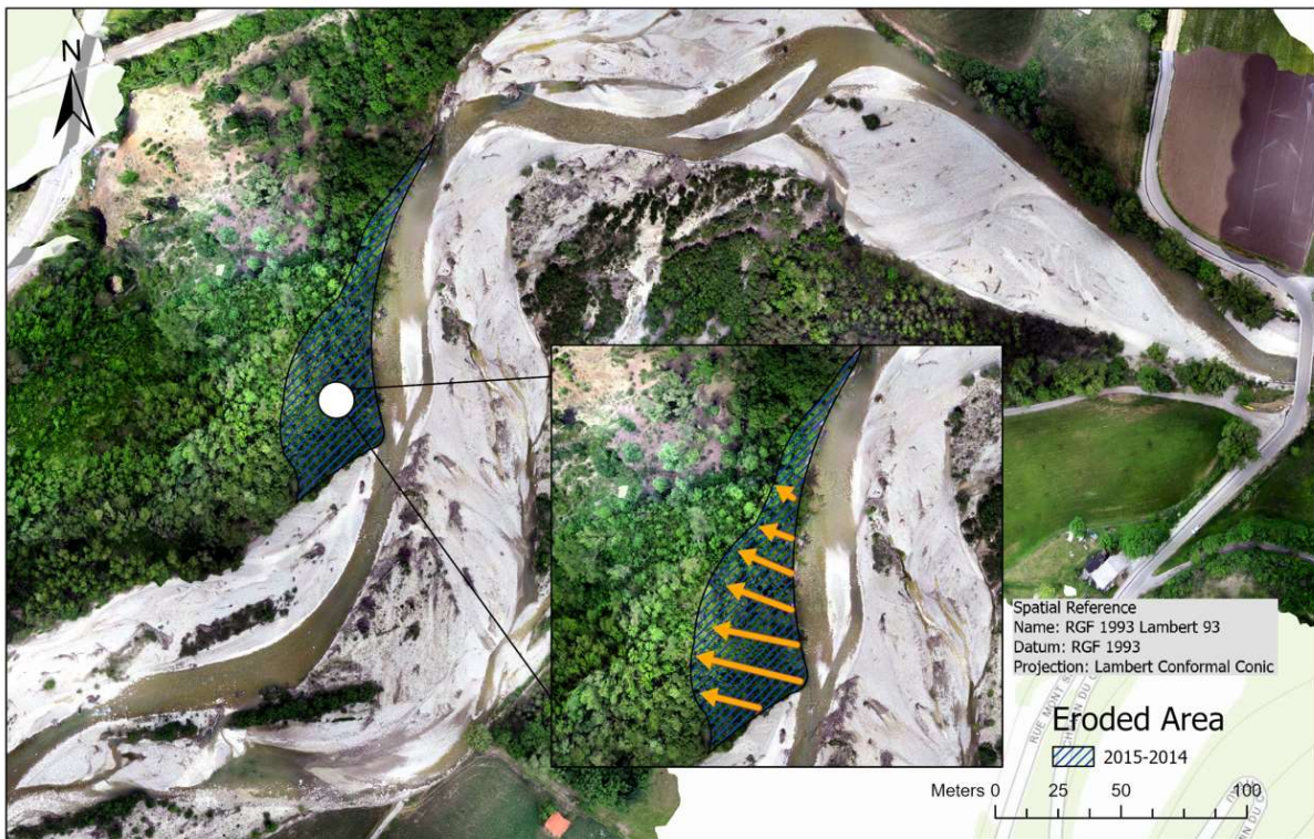
Figure 14 : Total eroded area between 2015 and 2014 , which is approximates 6040 m 3 .
