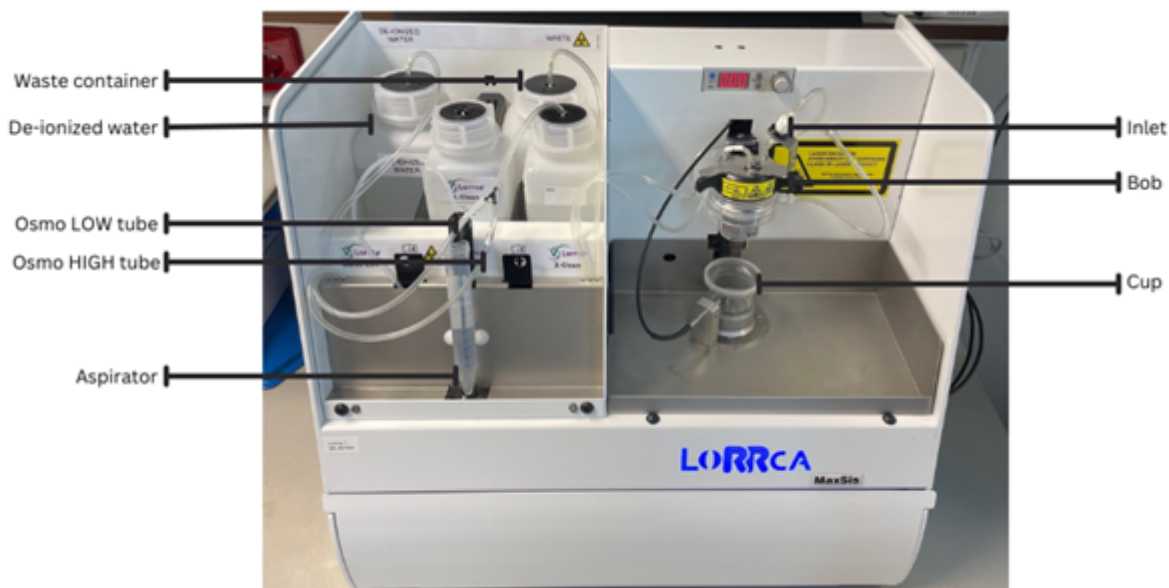
Figure 2.4 Set up of a Laser Optical Red Cell Analyzer (Lorrca MaxSis, RR Mechatronics, Zwaag, The Netherlands)
