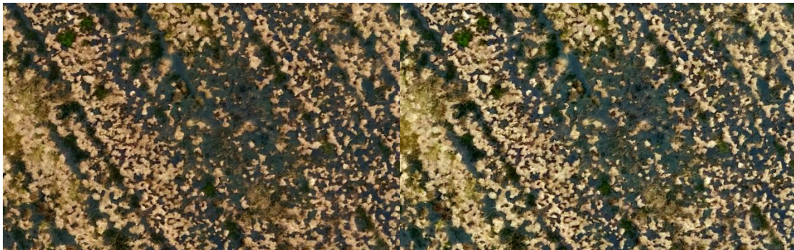
Fig 18. Section of Site C showing how the Minimum- Maximum stretch 2 increased the contrast of the RGB image (left).
