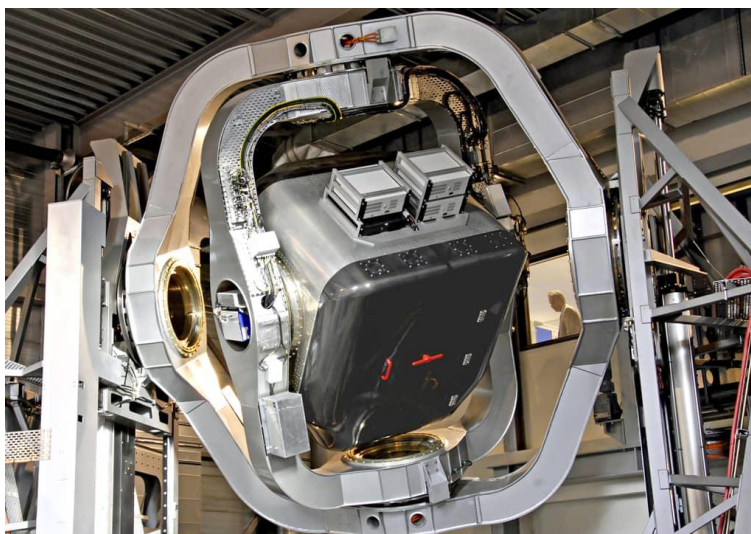
Figure 2. DESDEMONA Centrifuge-Based All-Attitude Simulator. Photo by (AMST, sd)
