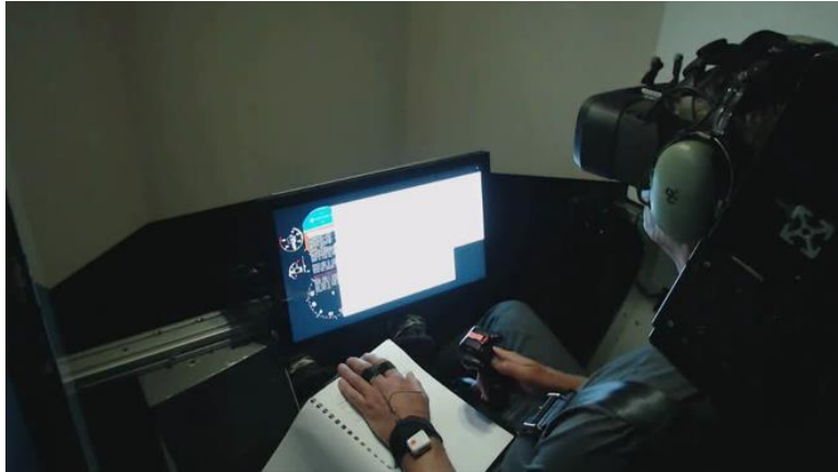
Figure 3. Participant in the DESDEMONA simulator, wearing the VARJO AERO, David Clark H10-13.4 and physiology sensors.
