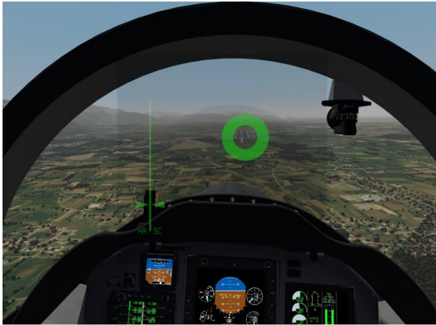
Figure 4. Participant's view within the simulation. The light grey square represents the HMD, with the biofeedback interface positioned on the left side. In this scenario, the biofeedback is deactivated and fixed at 20% of the display height. The green circle, which serves as an eye tracker (not visible to participants), is centered over the runway.
