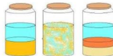
Figure 10 Soil composition test, (1) soil and water (2) mixture (3) 67% clay, 33% sand and water
