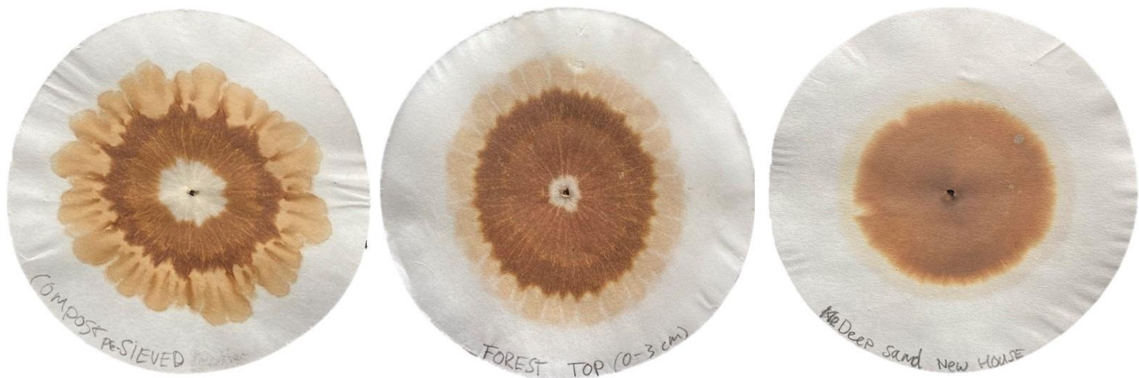
Figure 31 Pfeiffer chromatography samples used as references. Compost on the left as nutrient-rich, Forest top layer in the middle as healthy balanced reference and deep sand layer on the right as nutrient poor, unhealthy reference.
