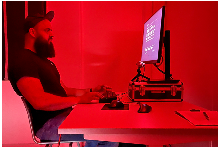
Figure 4.4: Photo to showcase the experimental setup, with the eye tracker placed beneath the screen slightly tilted upwards to capture the eyes and the red light. Noteworthy, for creating the picture extra daylight was let into the room.
