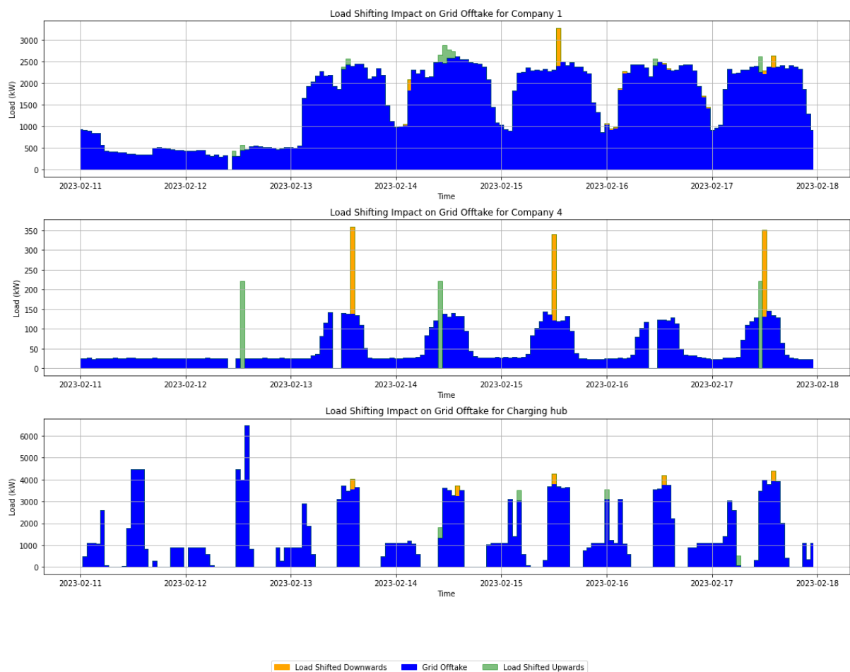
Figure 34: This graph shows the impact of upward and downward load shifting on the grid offtake. It shows data during the week of February 11 through 17. The charts mention 2023, but it should be 2040. This could not be changed; otherwise, the code would not work.
