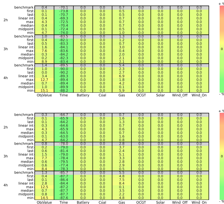
Figure 19: Overview of the results of the validation of the basic statistics methods in the investment model with climate year 1997 (top) and 2011 (bottom). On the x-axis the evaluation metrics are displayed including the objective value (total system cost), solve time and the investment decisions for generation and flexibility assets in the model. On the y-axis, the different down-sampling methods are displayed including the different resolutions. The numbers in the cells of the matrix indicate the percentage difference between the experiment and the hourly reference model. The benchmark is indicated in grey. Note that for the objective value and investment decisions the differences are absolute while for the solve time, they are not.
