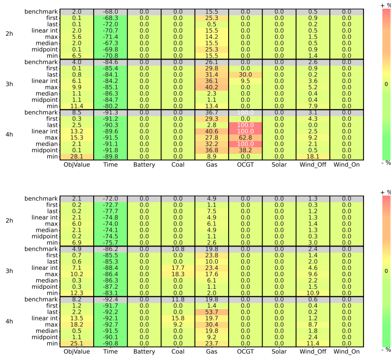
Figure 20: Overview of the results of the validation of the basic statistics methods in the increased limit investment model with climate year 1997 (top) and 2011 (bottom). On the x-axis the evaluation metrics are displayed including the objective value (total system cost), solve time and the investment decisions for generation and flexibility assets in the model. On the y-axis, the different down-sampling methods are displayed including the different resolutions. The numbers in the cells of the matrix indicate the percentage difference between the experiment and the hourly reference model. The benchmark is indicated in grey. Note that for the objective value and investment decisions the differences are absolute while for the solve time, they are not.
