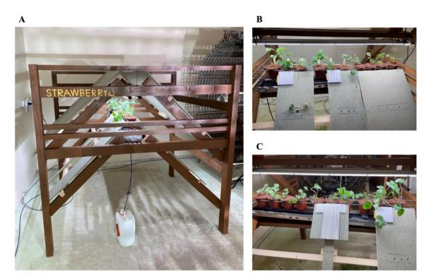
*Note.* (A) The wooden prototype was built based on the 3D model. (B) Two 3D printing bioinspired structures are attached to the panels. One is with gaps around 1 cm in width (left), and the other is with gaps around 2 cm in width (right). (C) Two control structures are placed on the panels. One is a combination of several L-shaped PVC (left) with one-centimeter-width gaps, and the other is a 3D printing V-shaped structure with gaps approximately 0.7 cm in width (right).
