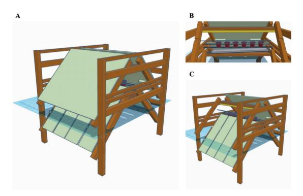
*Note*. (A) A prototype is sketched in a 3D model. The structure in brown is designated to be built in wood, the lines in black are for steel rods, and the green planes represent waterproof panels attaching the bio-inspired structure. (B) One row of strawberry plants can be grown in the middle of the prototype. (C) The panels are removable.
