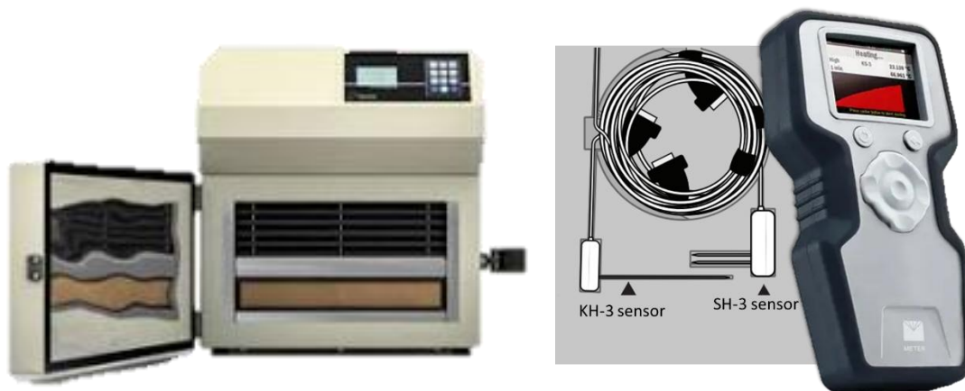
Figure 3. The heat flow meter (HFM-100) (a) and TEMPOS thermal properties analyzer (b).
