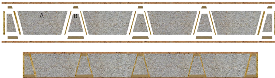
Figure 2. The cross-section view of Cir-Q. A is main filling, B is column filling.
