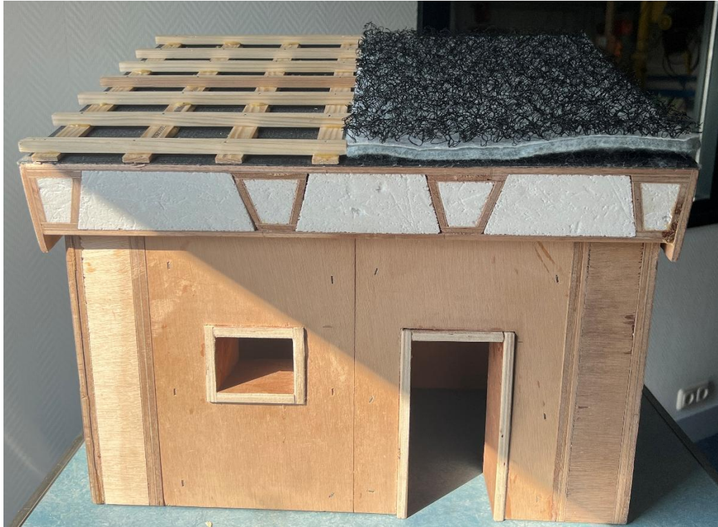
Figure 1. The prototype of a house made of Cir-Q. The prototype was made by Hans Borra.
