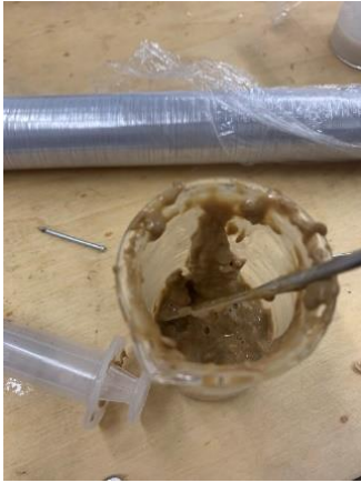
Figure 12: Mixing casein glue with wood saw dust.
