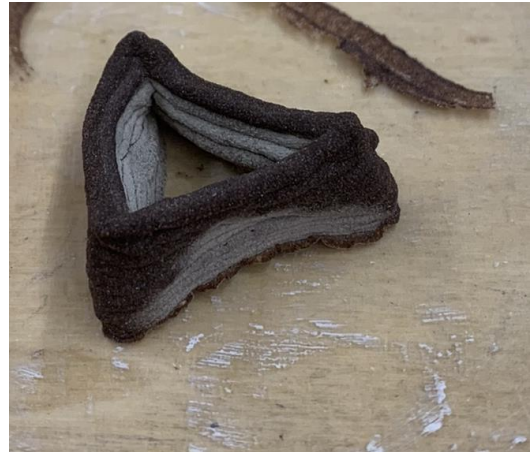
Figure 15: Print with printer of first casein glue / cork / oyster shell powder recipe (semi-dry)
