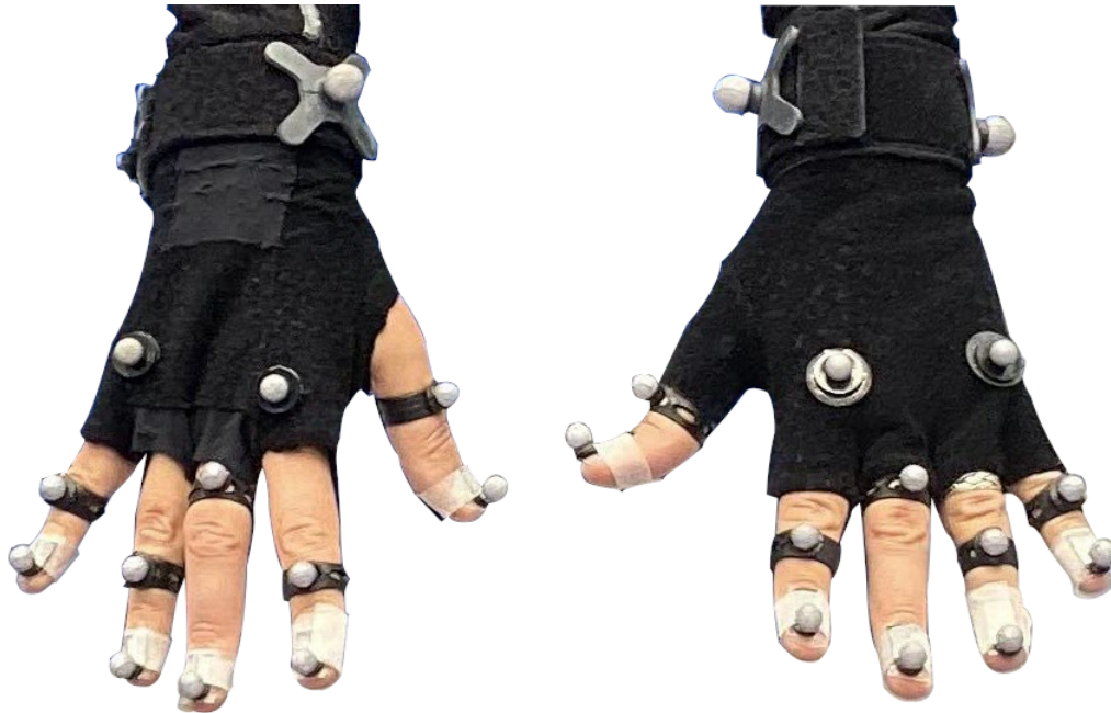
Figure 3: Placement for all the finger markers for the 10 finger marker set as depicted in Vicon documentation [25]
