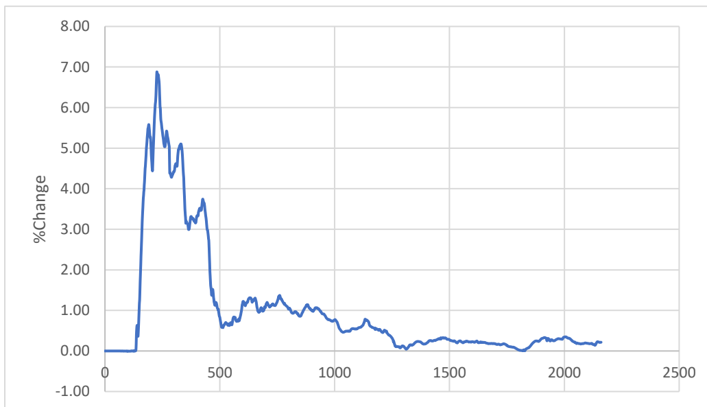
Figure 20: Percentage Change in Outlet Temperature Between High and Low Mesh Resolutions
